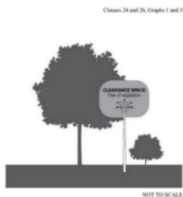
FIGURE 5 – UNINSULATED 66 000 VOLTAGE ELECTRICAL LINE IN A LOW BUSHFIRE RISK AREA AND UNINSULATED ELECTRIC LINE IN A HAZARDOUS BUSHFIRE RISK AREA
