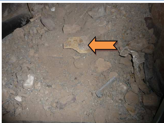
Photo 11. Main Building basement – Plant Area 2 – rubble - asbestos vinyl tile debris. Sample 19952-001-025A.
