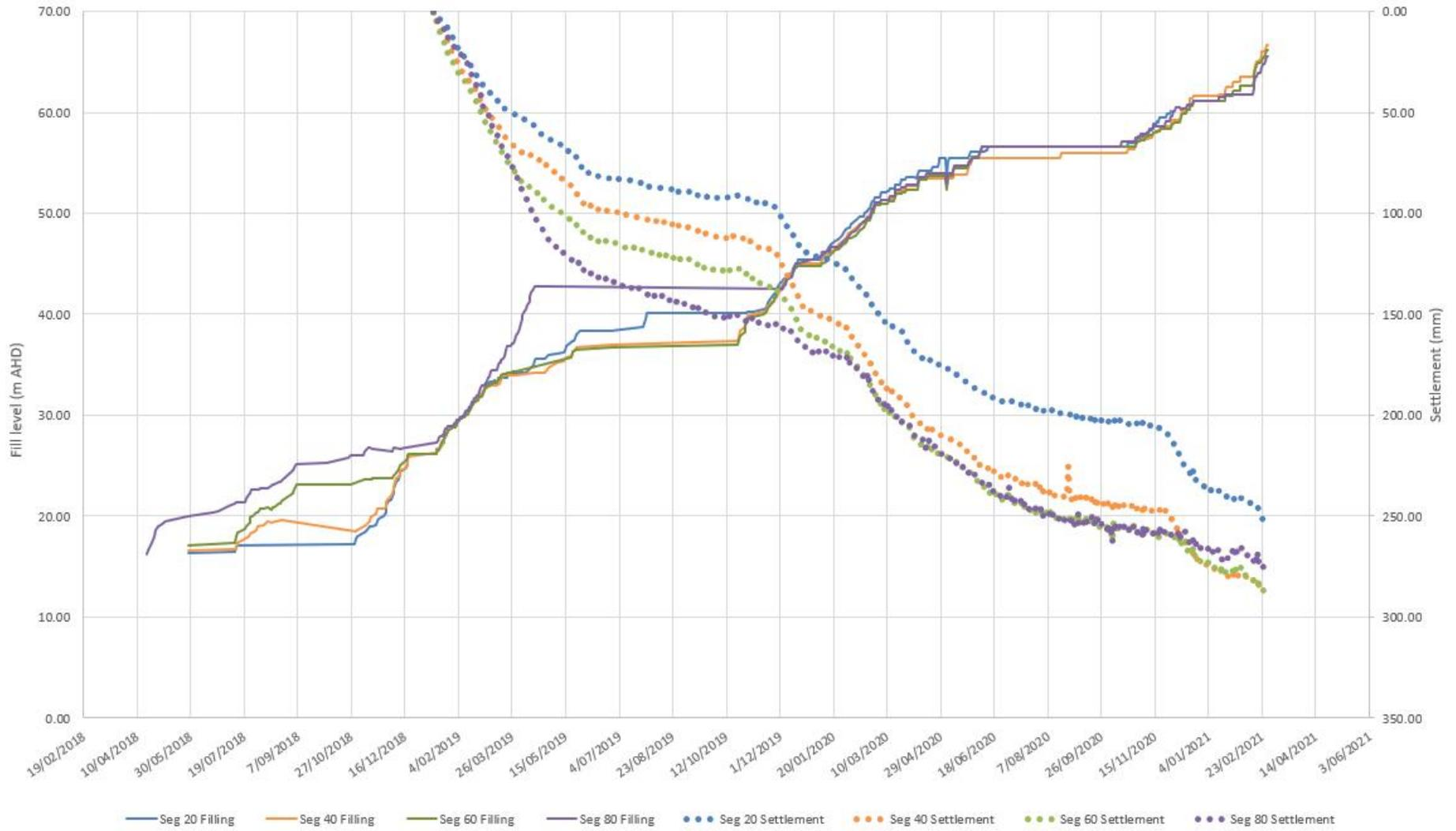
Plot of southern shape array settlement versus fill height above shape array
