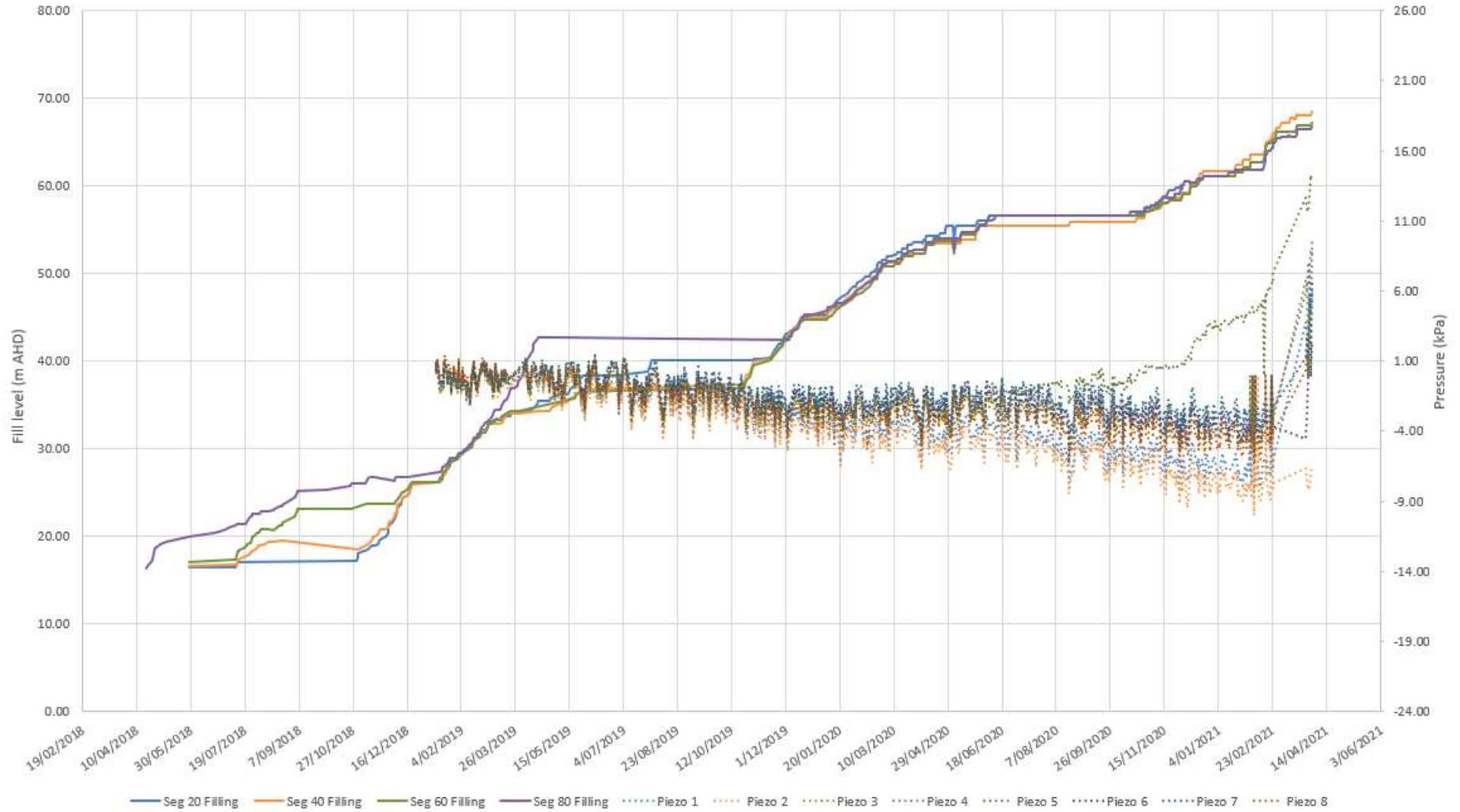
Plot of southern vibrating wire piezometers versus fill height above shape array
