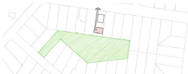
New dwellings (red) oriented to face park with low, semi-transparent front fences. Access for new dwellings backwards through driveway of existing dwelling and onto road. Parking for existing dwelling relocated to the rear
