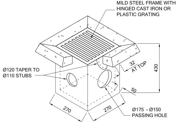
KNOCKOUT HOLE FORMERS LOCATED AT 20mm ABOVE INVERT. HOLES CAN BE RELOCATED TO INVERT REQUIREMENTS
